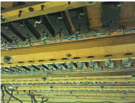
Organ mechanism underneath pipe chest
