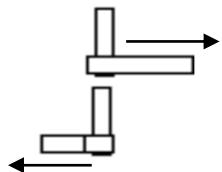
5. Bend the **top strip forward and put the end through the center square** to make a shaft of desired length.
