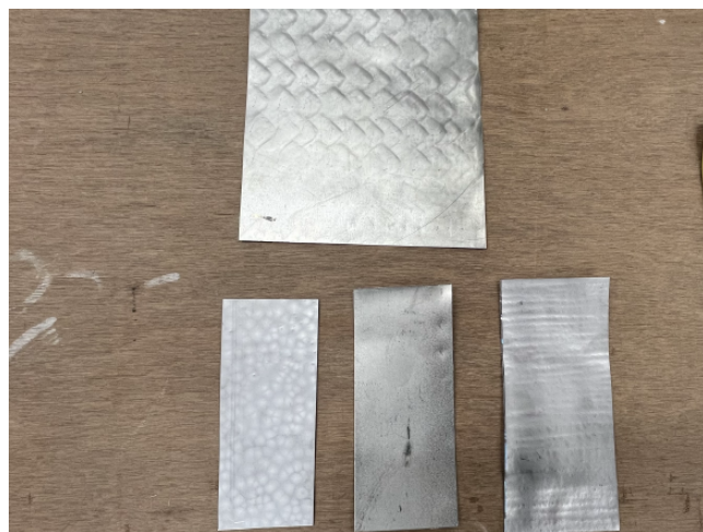
Various metal alloys. (Top) Hammered sheet (Bot. L-R) 50%, 90% tin, 97% lead
