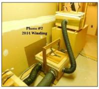
played and more wind is required. The <sup>3</sup>/<sub>4</sub> HP blower is no longer powerful enough for the reconfigured instrument. Photo #1 shows the winding in 1987. Photo #2 shows the winding in 2014. The story continues next week!
